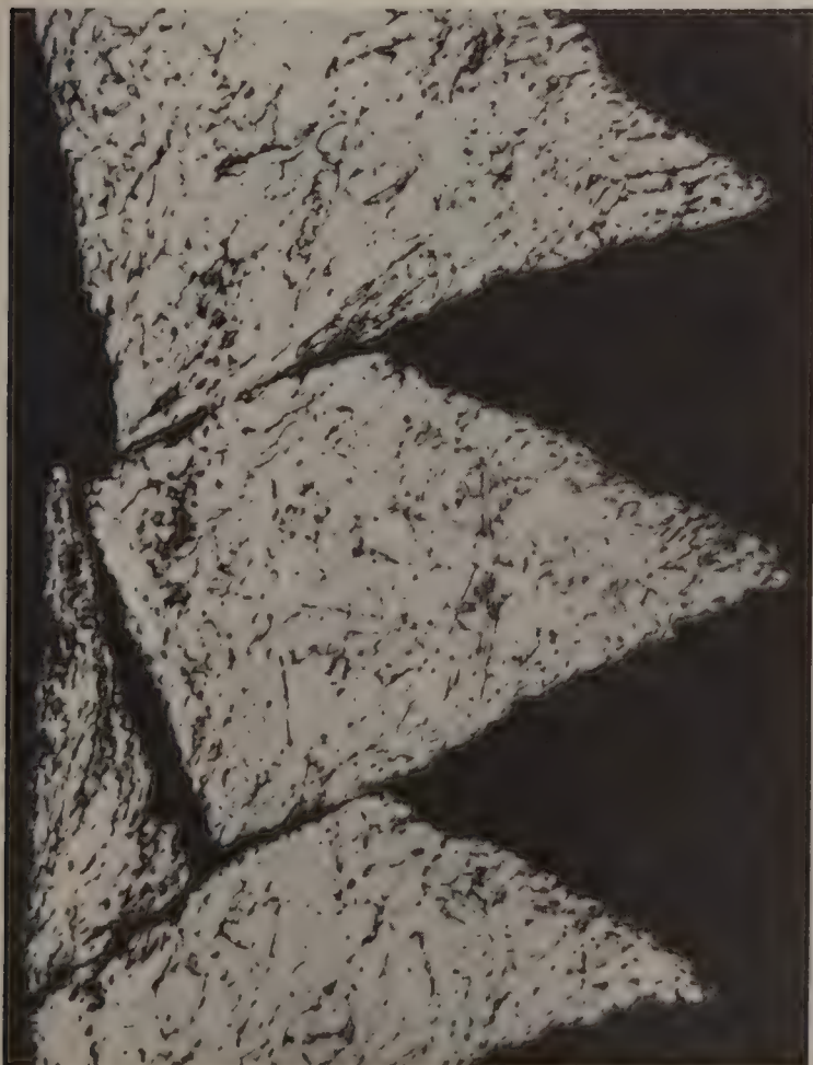
Fig. 9. Rewelded discontinuous titanium chip. Work material, Ti 75A cut at 1 in/min; 120x.
